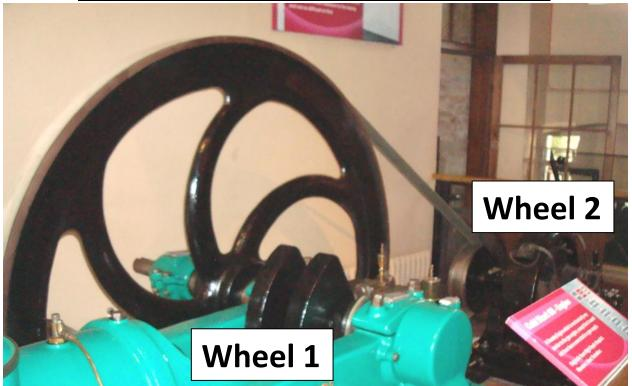
Wheel 2 is attached to wheel 1 by a belt, and for every **3 turns** of the large wheel makes, the small wheel goes round exactly **16 times**.
