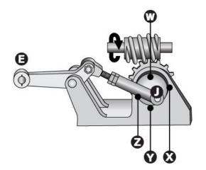
When the wheel turns, end E moves down and up in an arc. End E will be at the top of the arc when joint J is at point:
