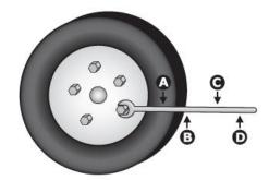
In which position should you hold the wrench in order to remove the lug nut with the least amount of force?
