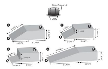
Which of the four platforms would require the least amount of force to roll the barrel from Point A to Point B?
