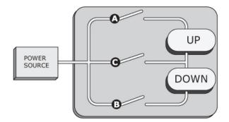
In order to activate the mechanism labelled "Up" without activating the mechanism labelled "Down", which combination of switches would need to be closed in the electrical circuit shown?
