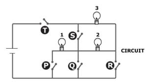
Which two switches should be closed to light up bulbs 2 and 3 only?
