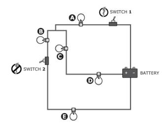
In the electrical circuit above, which light bulbs should be lit if Switch 1 is on and Switch 2 is off?
