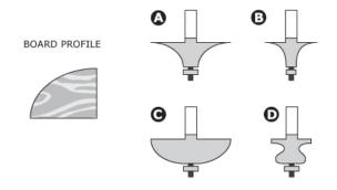
Which of the router bits would be most likely to reproduce the profile of the board shown?
