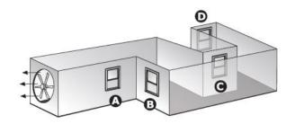
Which window should be opened to produce the greatest cooling potential for the entire house?
