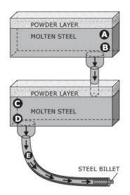
In the continuous casting system where molten steel is moving from Point A to Point E, at which point would the molten steel be the hottest and at which point would it be the coolest?
