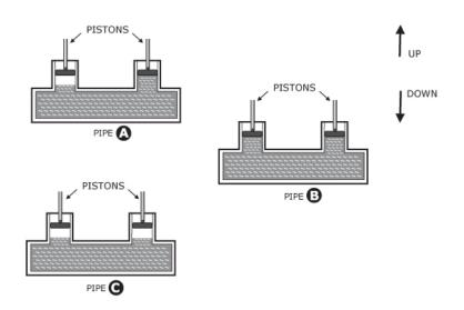
In the three hydraulic systems shown, if the left piston is pushed down equally, which of the following is true?
