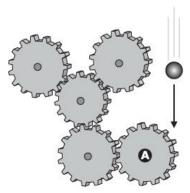
If a ball is dropped on Gear A at the specified point, how many gears will turn counterclockwise, assuming the force applied by the ball is sufficient to move all the gears?
