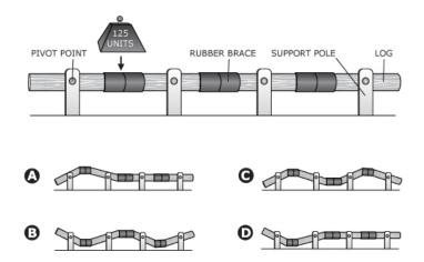
The image is of a series of logs held together by support poles (each with a pivot point) and by rubber braces which flex and bend. Which image would be the most likely result if the weight is placed on the rubber brace as pictured?
