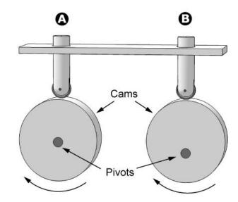
Which rod will move up and down more with one revolution of the cam?
