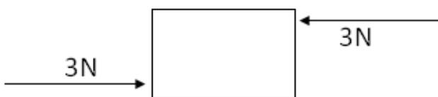
In this diagram, the resultant force is zero, since the only forces acting are balanced. However, the body is not in equilibrium because the moment is not zero.
