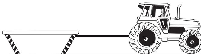
Assume that only **two** horizontal forces act on the tractor. One is a driving force, which has magnitude  $P$  newtons and acts in the direction of motion. The other is the tension in the rope.
